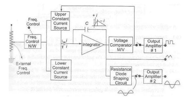
The block diagram of a function generator:
