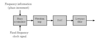
DDS frequency synthesizer as used in an arbitrary function generator, AFG
