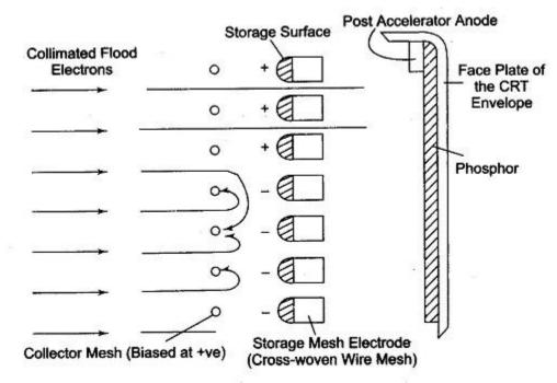
Figure 7.28 shows a display of the stored charge pattern on mesh storage.
