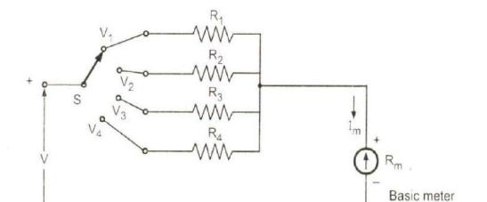
The R1, R2, R3 and R4 are the four series multipliers. When connected in series with the meter, they can give four different voltage ranges as V1, V2, V3, and V4. The selector switch S is multiposition switch by which the required multiplier can be selected in the circuit.
