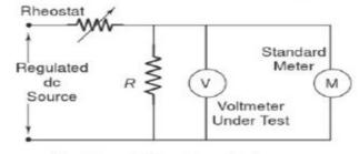
Fig. Calibration of voltmeter
