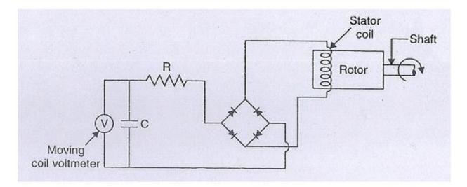
It consists of, like an alternator, a stationary armature (stator) and a rotating field system (rotor). Owing to the generation of e.m.f in a stationary coil on a stator, commutation problems no longer exist. The alternating e.m.f. induced in the stationary coil is rectified, and the output D.C. voltage is measured with the help of a moving coil voltmeter (V).
