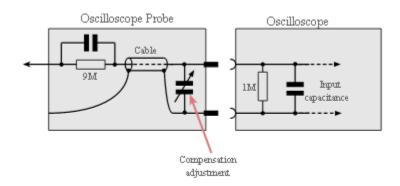
Oscilloscope probe circuit
