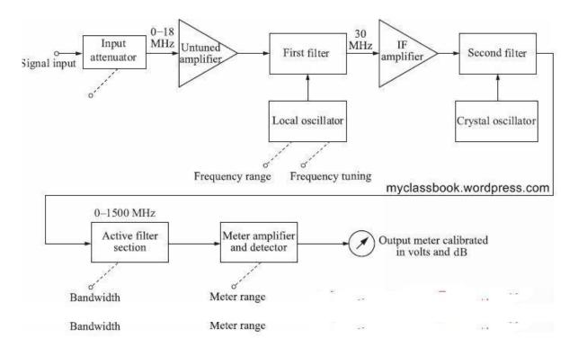
The block schematic of the wave analyser using the heterodyning principle is shown in fig. above. The operating frequency range of this instrument is from 10 kHz to 18 MHz in 18 overlapping bands selected by the frequency range control of the local oscillator. The bandwidth is controlled by an active filter and can be selected at 200, 1000, and 3000 Hz.
