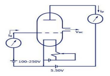
The grid is maintained at a large positive potential with respect to the cathode and the plate. The plate is at a negative potential with respect to the cathode. This method is also known as the external control type ionization gauge as the positive ion collector is external to the electron collector grid with reference to the cathode. The positive ions available between the grid and the cathode will be drawn by the cathode, and those between the grid and the collected by the plate.
