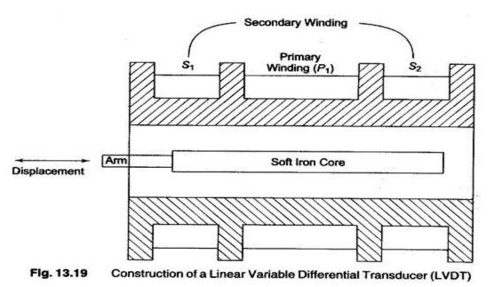
• The <u>transformer</u> consists of a single primary winding  $P_1$  and two secondary windings  $S_1$  and  $S_2$  wound on a hollow cylindrical former. The secondary windings have an equal
