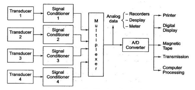
A typical <u>Data Acquisition System</u> consists of individual sensors with the necessary signal conditioning, data conversion, data processing, multiplexing, data handling and associated transmission, storage and display systems.
