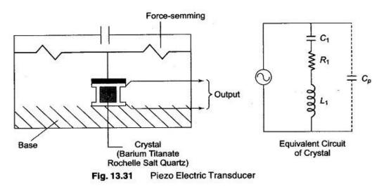
For a Piezoelectrical Transducer element under pressure, part of the energy is, converted to an <u>electric potential</u> that appears on opposite faces of the element, analogous to a charge on the plates of a capacitor. The rest of the applied <u>energy</u> is converted to mechanical energy, analogous to a compressed spring. When the pressure is removed, it returns to its original shape and loses its <u>electric charge</u>.
