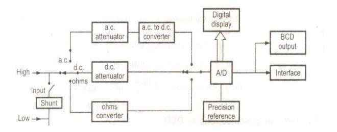
The current is converted to voltage by passing it through low shunt resistance. The a.c. quantities are *converted* to d.c. by employing various rectifier and filtering circuits. While for the resistance measurements the meter consists of a precision low current source that is applied across the unknown resistance while gives d.c. voltage. All the quantities are digitized using analog to digital
