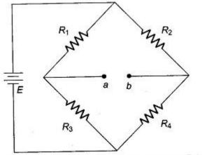
Fig. 11.2 Unbalanced Wheatstone's Bridge
