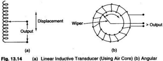
Inductive Transducer (Using Ferrite Core)
