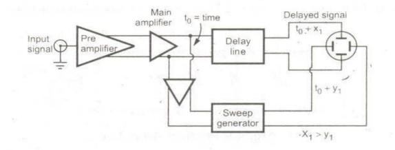
If the trigger pulse is picked off at a time t = to after the signal has passed through the main amplifier then signal is delayed by XI nanoseconds while sweep takes YI nanoseconds to reach. The design of delay line is such that the delay time XI is higher than the time YI' Generally XI is
