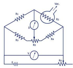
When the pressure changes, there will be a change in current. For this, the voltage V has to be kept constant. The resistance R2 of the gauge is measured, by keeping the gauge current constant. The null balance of the bridge circuit is maintained by adjusting the voltage or current. This change is made with the help of a potentiometer and the change brought will be a measure of the pressure produced.
