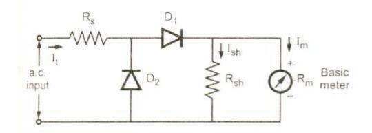
The diodes D1 and D2 are used for the rectifier circuit. The diodes show the nonlinear behaviour for the low currents hence to increase the current through diode D1, the meter is shunted with a resistance Rsh' This ensures high current through diode and its linear behaviour.
