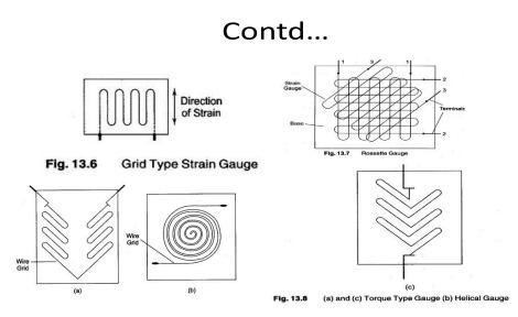
Characteristics of a resistance wire strain gauge
