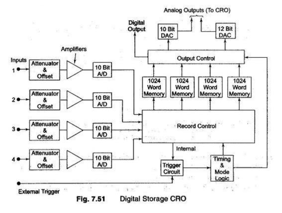
The analog input voltage is sampled at adjustable rates (up to 100,000 samples per second) and data points are read onto the memory. A maximum of 4096 points are storable in this particular instrument. (Sampling rate and memory size is selected to suit the duration and waveform of the physical event being recorded.)
