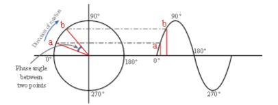
Phase angle of points on a sine wave
