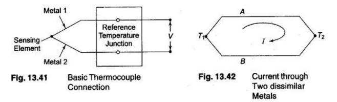
A current will circulate around a loop made up of two dissimilar metal when the two junctions are at different temperatures. When this circuit is opened, a voltage appears that is proportional to the observed seeback current. The Thomson and Peltier emfs originate from the fact that, within conductors, the density of free charge carriers (electrons and holes) increases with temperature.
