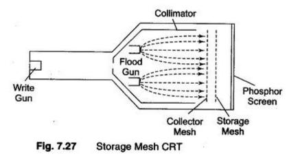
Since the storage mesh makes use of secondary emission, between the first and second crossover more electrons are emitted than are absorbed by the material, and hence a net positive charge results.
