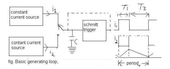
The upper current source supplies a constant current to the capacitor and the capacitor voltage increases linearly. When the positive slope of the ramp voltage reaches the upper limit set
