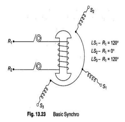
The rotor is energized by an ac voltage and coupling between rotor and stator windings varies as a trigonometric or <u>linear function</u> of the rotor position.
