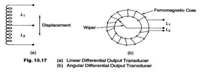
Linear Variable Differential Transducer (LVDT)
