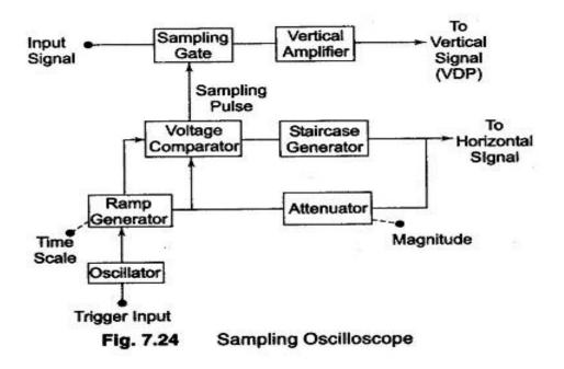
Figure 7.24 shows a block diagram of a sampling oscilloscope. The input waveform is applied to the sampling gate. The input waveform is sampled whenever a sampling pulse opens the sampling gate. The sampling must be synchronised with the input signal frequency. The signal is delayed in the vertical amplifier, allowing the horizontal sweep to be initiated by the input signal. The waveforms are shown in Fig. 7.25.
