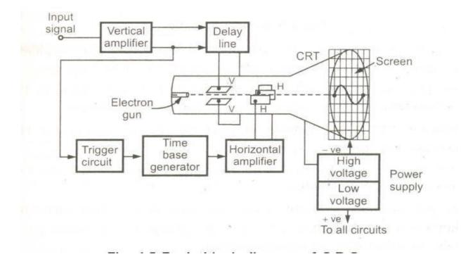
This is the cathode ray tube which is the heart of CR.O. It is' used to emit the rlectrons required to strike the phosphor screen to produce the spot for the visual display of the signals.
