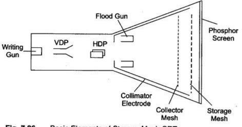
Fig. 7.26 Basic Elements of Storage Mesh CRT
