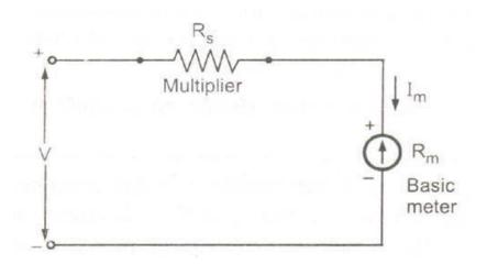
The voltmeter must be connected across the two points or a component, to measure the potential difference, with the proper polarity.
