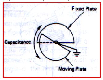
It consists of a fixed cylinder and a moving cylinder. These pieces are configured so the moving piece fits inside the fixed piece but insulated from it.
