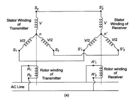
(a) Torque Transmission Using Synchro Trans
