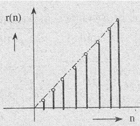
fig 7.2 (b) Discrete Ramp Signal
