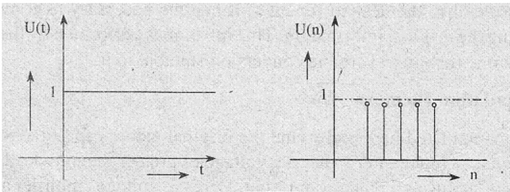
fig 7.1 (a) Continuous Time Step Input
