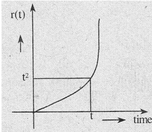
fig 7.3 (a) Unit Parabolic Signal
