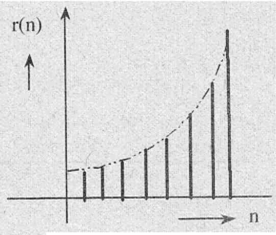
fig 7.3 (b) Discrete Parabolic Signal
