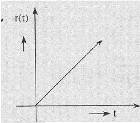
fig 7.2 (a) Unit Ramp Signal
