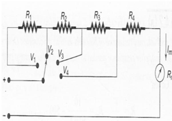
fig 4.3 Multiplier connected in series string
