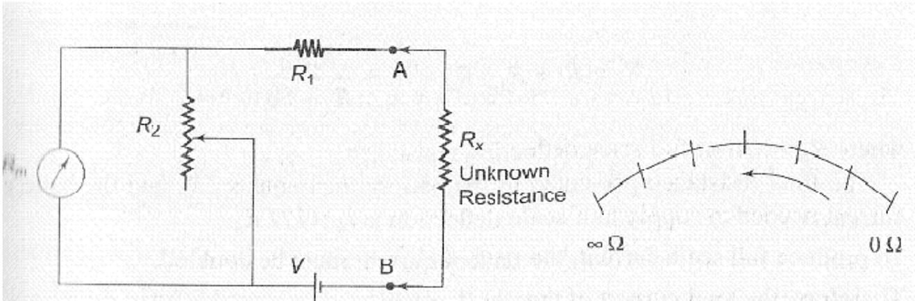
fig 11.1 Series type ohm meter
