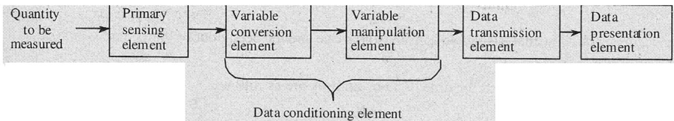
fig 6.1 Functiona Elements of measuring sysstem
