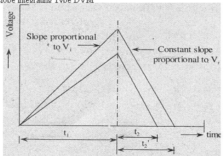
fig 10.2 Basic principle
