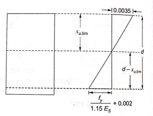
$$\frac{d}{x_{\text{II}, \text{lim}}} = \frac{0.0055E_{\text{s}} + 0.87 \, f_{\text{y}}}{0.0035 \, E_{\text{s}}} \qquad [E_{\text{s}} = 2 \times 10^{5} \, \text{N/mm}^{2}]$$
