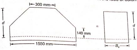
Here b = 300 mm, B = 1550 mmWidth of equivalent section,
