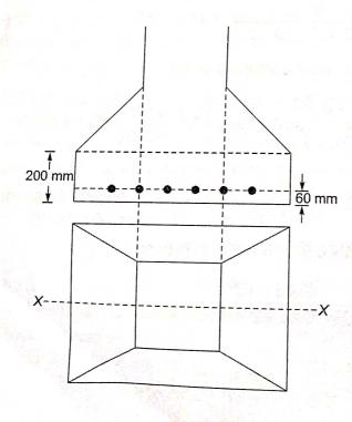
Assuming depth of slab = 200 mm and nominal cover = 60 mm Depth of foundation for bending moment critical section is at the face of column section
