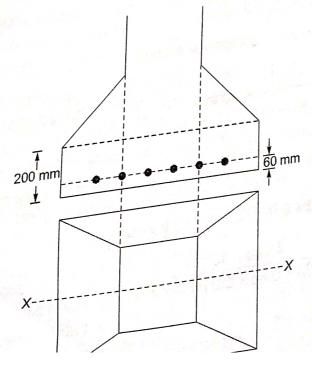
Assuming depth of slab = 200 mm and nominal cover = 60 mm Q.25 Design a sloped square footing of a RC column 300 mm imes 300 mm size carrying an axial load of 320 kN. The safe bearing capacity of soil is 150 kN/m². M20 concrete and Fe 415 steel are used. Use working stress method of design.
