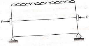
Due to this prestressing force, the compressive stress induced in concrete =  $f_a = \frac{P}{A}$  where A is the
