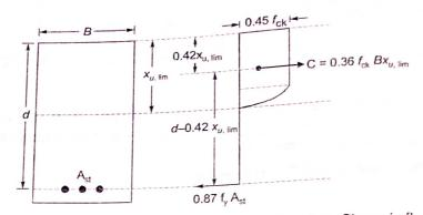
Limiting percentage of tensile steel is calculated for a balanced section. Since, in flexure total compressive force is equal to total tensile force, we get
