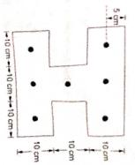
Area of cross section,  $A = 300 \times 300 - 2 \times 100 \times 100 = 70,000 \text{ mm}^2$
