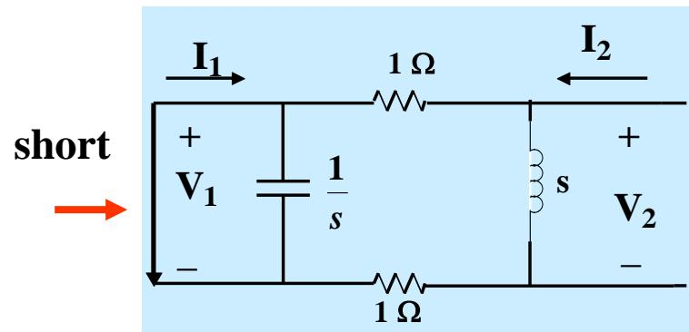
$$y_{22} = \frac{I_2}{V_2} \quad | \quad V_1 = 0$$
