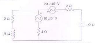
Find the voltage drop across the capacitor using superposition theorem.
