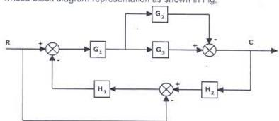
Determine the transfer function(C/R) of the system shown in Fig,using Mason's Gain Formula.
