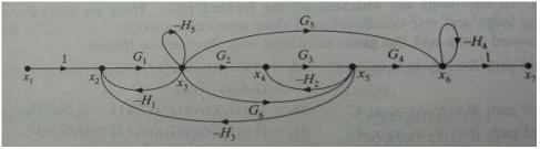
Using mason gain formula find the transfer function  $\overset{\textbf{C}}{\text{for the signal flow graph}}$  shown in figure.
