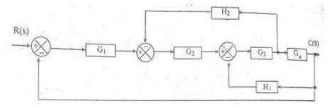
Find the overall transfer function of the system whose signal flow graph is shown below.
