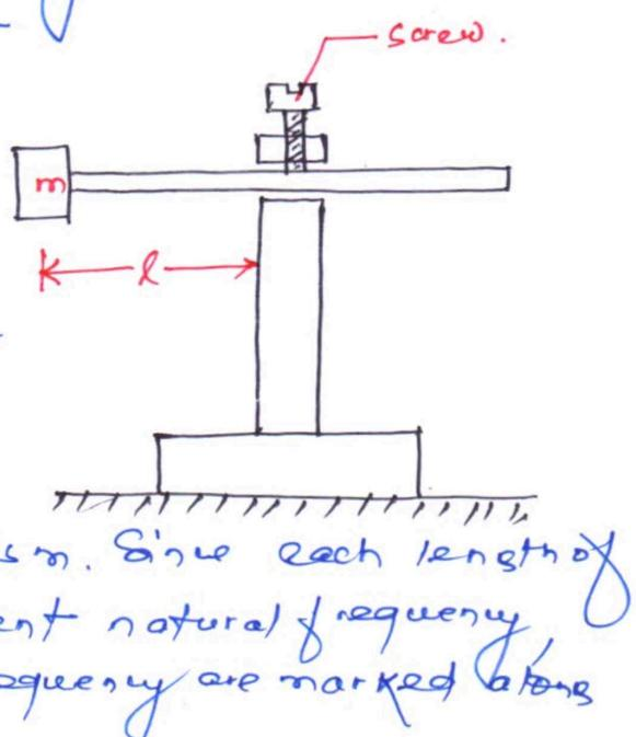
means of screw mechanism. Since each length of strip corresponds to a different natural frequency, so the values of natural frequency are marked along
