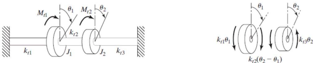
Figure 2 Torsional vibration of a two rotor system
