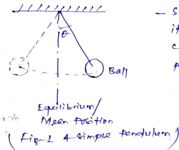
— So any motion which repeats itself after an interval of time is called vibration; e.g. simple pendulum (shown in fig-1)
