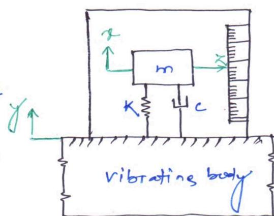
The arrangement is similar to the spring-mass-dashpot system having support. The displacement of the mass relative to the box i.e. 'x' can be measured by attaching a pointer to the mass and a scale to the box.
