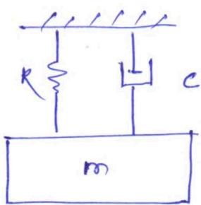
In the study of vibration, the process of energy dissipation is generally referred to as damping. The most common phenomenon of energy dissipating element is viscous damper, also called dashpot.
