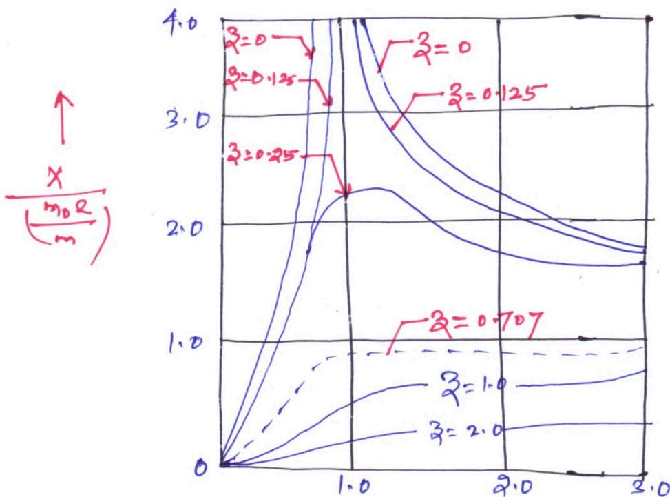
( Dimensionless amplitude  $\left(\frac{\omega}{\omega_n}\right)$  frequency ratio plot )
