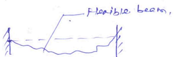
(Fig. 6: A flexible beam having infinite dof)
