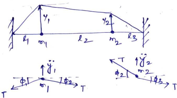
consider two masses fixed on a tight string stretched between two supports and having tension  $T$ . Let the amplitude of vibration is small and tension  $T$  is large.
