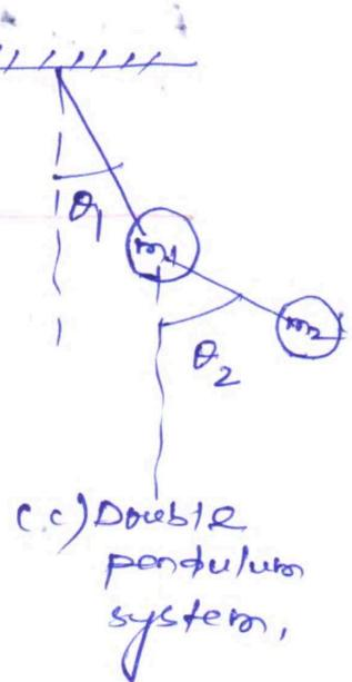
(Fig 3:- Examples of two degrees of freedom (DOF) systems)
