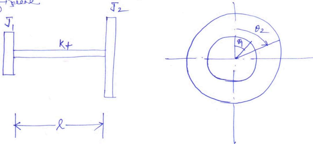
Let \$J\_1, J\_2\$ = moment of inertia of rotor 1 and rotor 2 respectively
