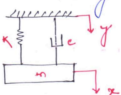
considering a spring-mass-damper system the mass is attached with the support by means of a spring of stiffness  $K$ , a damper of damping coefficient  $c$ .
