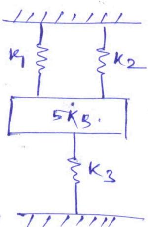
The equivalent stiffness for springs in parallel
