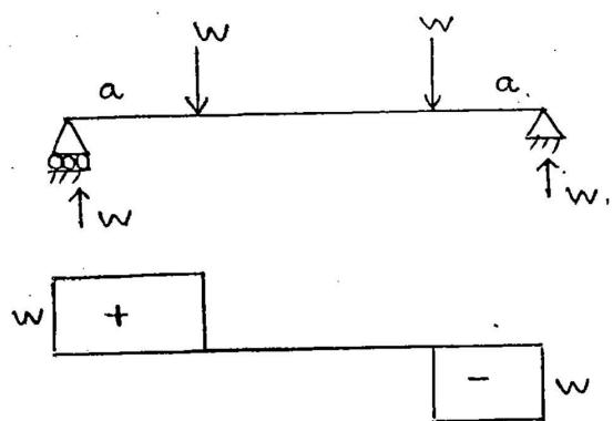
In laboratories, we apply two-point load systems. It is done to eliminate shear and obtain pure bending criterion. Cracks formed will be due to bending - flexural crack
