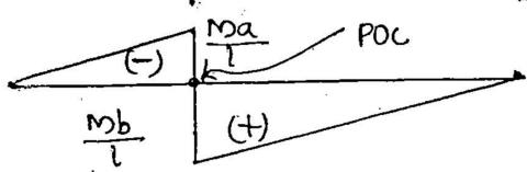
**Point of Contraflexure:** Point where bending moment changes sign, or curvature of the beam reverses its direction.
