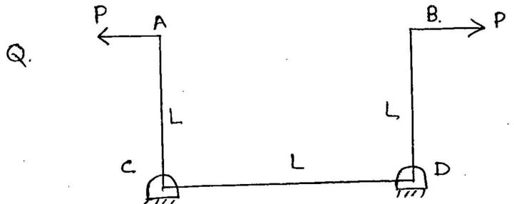
Determine relative displacement between A & B.
