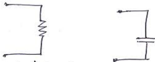
Two port Network → The n/w having two pairs of terminal or four terminals is known as two port n/w.
