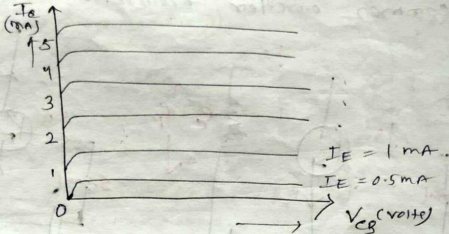
→ It is the curve between collector current  $I_c$  and collector-base voltage  $V_{CB}$  at constant emitter current  $I_E$ .
