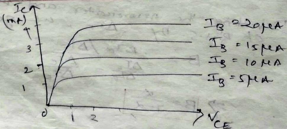
→ It is the curve between collector current  $I_c$  and collector-emitter voltage  $V_{CE}$  at constant  $I_B$ .
