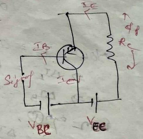
→ In this circuit arrangement, r/p is applied between base and collector while o/p is taken between the emitter and collector.
