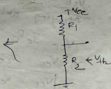
$V_{th}$  = Thevenin voltage = the potential across  $R_2$  (lower resistance)
