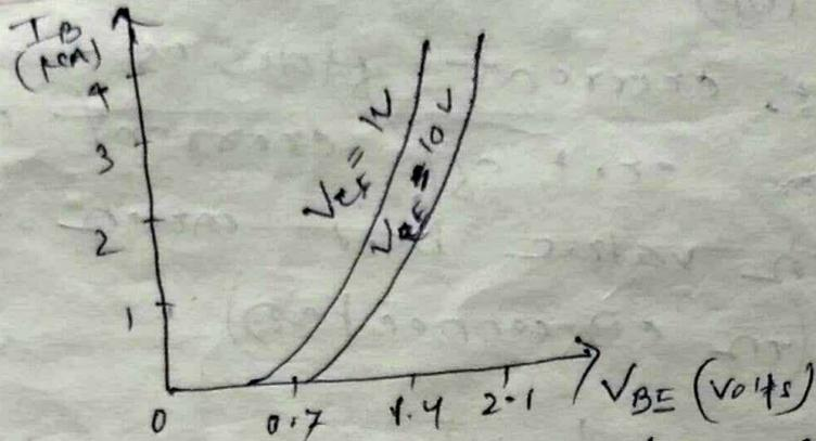
→ It is the curve between base current  $I_B$  and base-emitter voltage  $V_{BE}$  at constant collector-emitter voltage  $V_{CE}$ .
