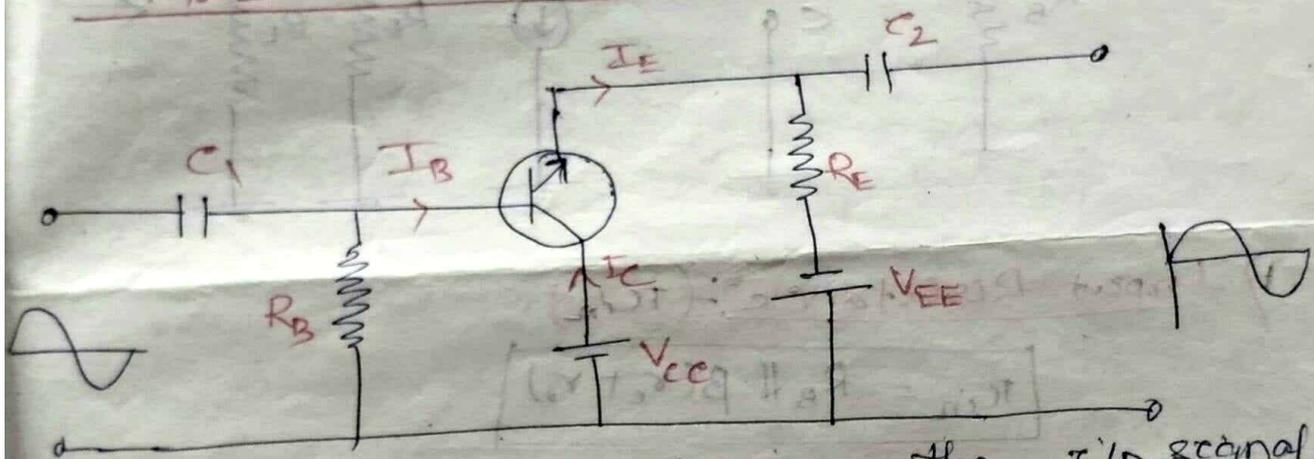
→ In the CC amplifier, the i/p signal is applied across B/C junction & o/p signal is taken out from E/C junction.
