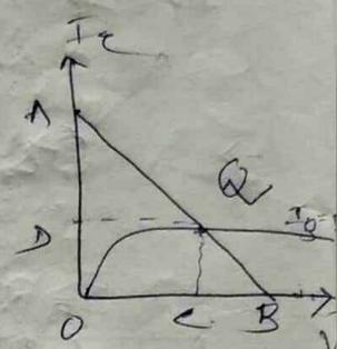
→ Again we require two end points, one maximum collector-emitter voltage point  $(V_{CE})$  the other is maximum collector current point  $(I_C)$
