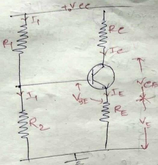
→ In this method  $R_1$  and  $R_2$  resistors are connected from  $V_{cc}$  to ground in such a way that the total voltage is divided into two parts from which the lower part is applicable for biasing.
