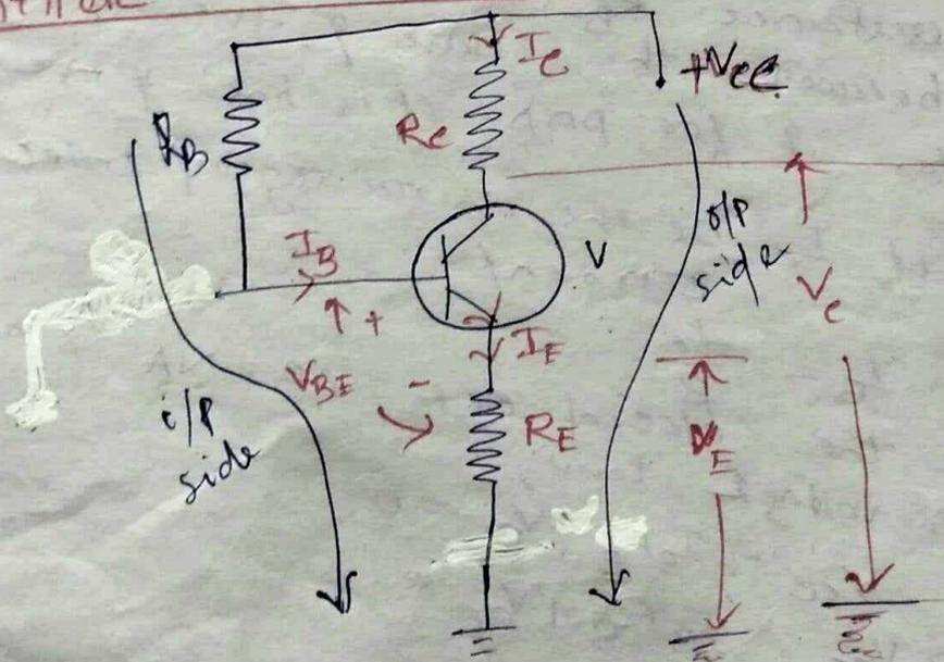
→ Here, an emitter resistor ( $R_E$ ) is present across the emitter terminal as shown in the figure.
