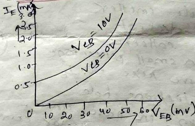
→ It is the curve between emitter current  $I_E$  and emitter-base voltage  $V_{EB}$  at constant collector-base voltage  $V_{CB}$ .
