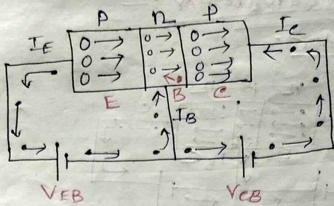
→ The forward bias causes the holes in the p-type emitter to flow towards the base and that constitute emitter current  $I_E$ .
