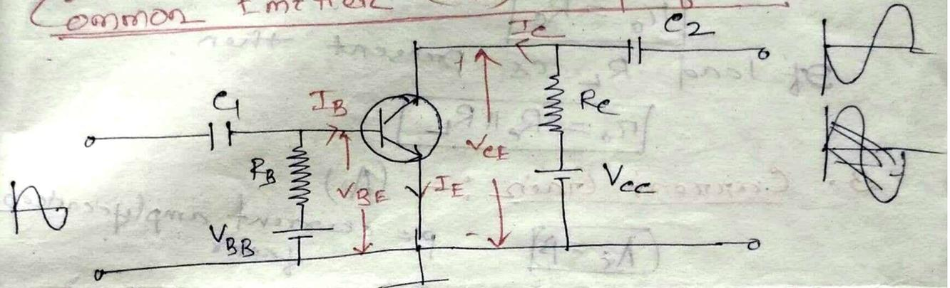
→ Here, i/p signal is injected into the B/E ckt and o/p is taken from C/E junction, of a NPN transistor.
