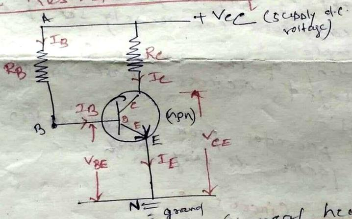
→ A high resistance  $R_B$  (several hundred  $k\Omega$ ) is connected between the base & +ve end of supply for npn ts. & for pnp it is base & -ve supply end.
